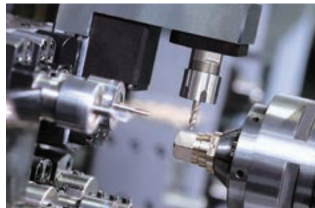
選配：背面選配Y2軸時可加選配立式鑽銑刀具刀座 Option: Optional Radial drilling tool holder when Y2 axis is selected on the sub-spindle
