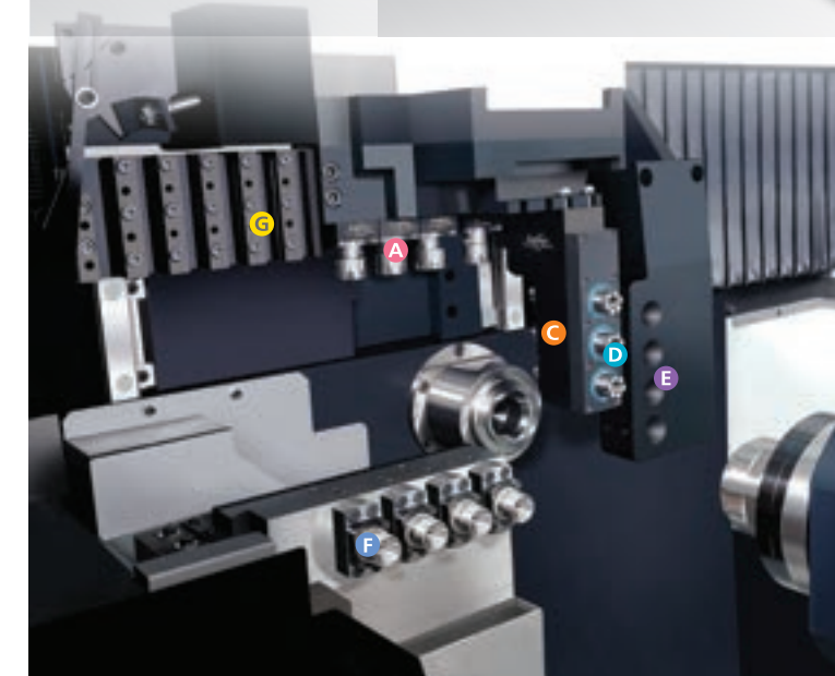
Using Live Bushing with Guide Bush 有導套之主軸構造
