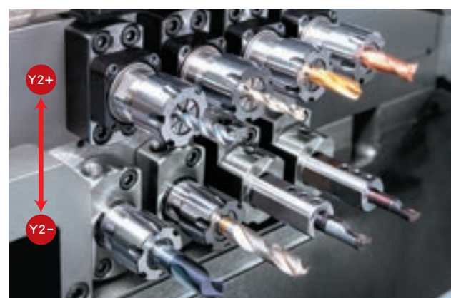
選配：背面Y2軸 Option: Sub-spindle has Y2 axis
